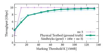
Figure 1: Throughput for two dctcp flows in ns-3, a physical testbed, and a SimBricks end-to-end simulation.
