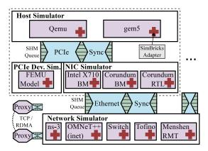
Figure 3: SimBricks architecture. *Double hour glass* with narrow waists between hosts and devices, and NICs and networks.
